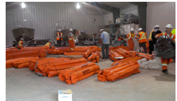
Additional Booms for River Spill Response Churchill Falls.
