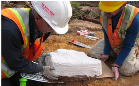
Recovery method referred to as a "block-lift" where the entire block of sand is excavated in the laboratory, due to the fragility of the artifacts.
